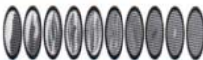
The above figure shows a spiral mixer, blending a black with white epoxy, in a series of 10 spiral-mixing elements. Note the striations.
